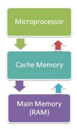
It is a **volatile memory**. It means it does not store data or instructions permanently. It is read/write memory which stores data till the machine is working. When you switch on the computer and perform some task the data and instructions from the hard disk are stored in RAM.
